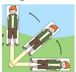
Lever- a bar which turns around a point/pivot.
